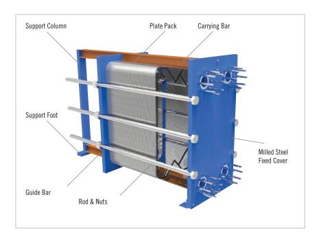
The most common material for the plates is 304 or 316 stainless steel in a (.4mm), (.5mm) or (.6mm) thickness. Gaskets type depends on the operating application, typically Buna (NBR/Nitrile), EPDM or Viton elastomer gaskets are usually specified.
