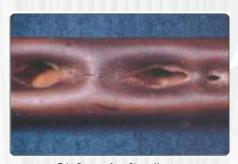
Tube Damage from Steam Hammer
