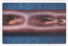
Tube Damage from Steam Hammer
