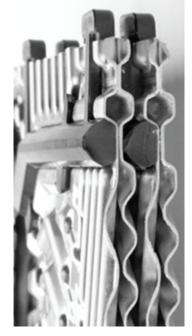
GASKETS ARE DESIGNED WITH VENTING PORTS, THESE PORTS PREVENT CROSS CONTAMINATION INSIDE THE HEAT EXCHANGER. WHEN A GASKET FAILS, THE LEAK IS DETECTED ON THE OUTSIDEOF THE PLATE PACK
