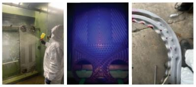
After being chemically cleaned, plates are high pressure washed and then plates are hung and sprayed with UV dye. Once sprayed the UV dye is allowed to soak in for 5 to 10 minutes and then using ultraviolet lights plates are inspected in a dark room for cracks, pin holes and deterioration. Any plates that are suspected of failure are then red/white dye penetrant tested so that failure can be confirmed.
