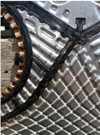
Hardened & Compacted Gasket
