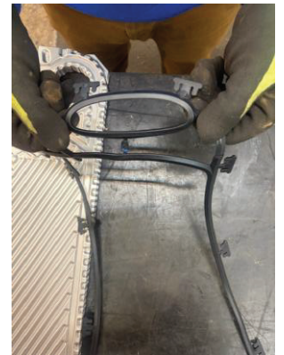
Gasket Quality Control: Tug Test & Inspection for defects
