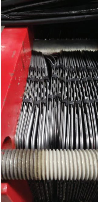
0.4mm Plate Pack Deformed & Misaligned
