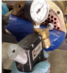
Brazed plate borescope inspection/ Brazed plate pressure test/ Acid flushing & filtering.
