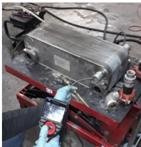
Brazed plate borescope inspection/ Brazed plate pressure test/ Acid flushing & filtering.
