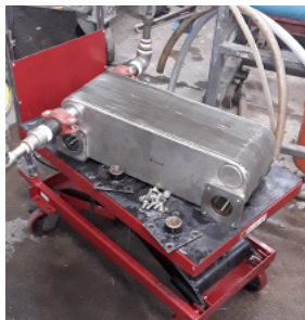
Brazed plate borescope inspection/ Brazed plate pressure test/ Acid flushing & filtering.
