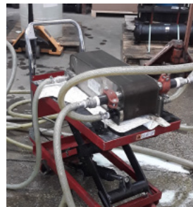
Brazed plate borescope inspection/ Brazed plate pressure test/ Acid flushing & filtering.
